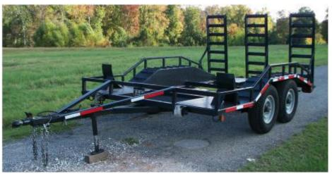
The Three Wheel Lift Transport trailer was designed to move 3-wheel lift machines for the poultry industry. The three wheel lift transport makes it easy to deliver an additional lift on site or to another location at a moments notice. Weight with BC3-5000 10,000 lbs. Capacity: 12,000 lb. GVWR.
