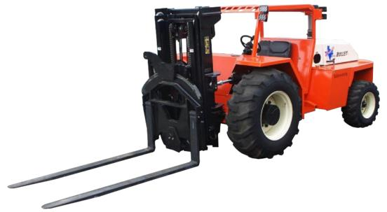
BASIC RATED CAPACITY: 6,000 lbs. @ 24"load center / 3,600 lbs. @ 48"load center
