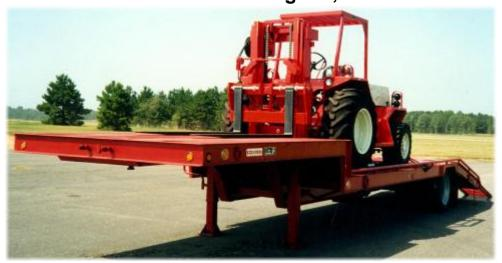
The Single Lift Transport trailer was designed to move 4-wheel lift machines for the poultry industry. The single lift transport makes it easy to deliver an additional lift on site or to another location at a moments notice. Capacity: 26,000 lb. GVWR.
