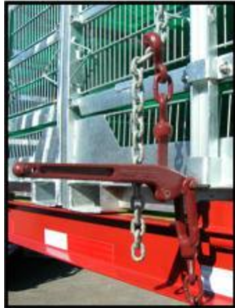
Picture shows chain loop being used to secure the binder to a tie bar beneath the trailer.
