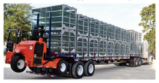
The poultry special double drop is designed solely for the addition and use of a 3-wheel lift. The ability to haul cages and a lift makes this complete package a must have in the poultry industry. Capacity: 80,000 lb. GVWR.
