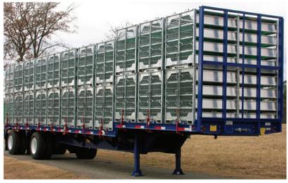
Designed specifically for the poultry industry. The Viking Specialized Poultry Platform Drop Deck is a poultry live transport trailer designed for chickens and turkey. Available front and rear bulkheads provide added security for cage movement and panels can be added to block direct wind during transportation. Capacity: 80,000 lb. GVWR.
