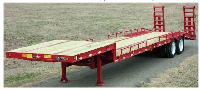
The Two Lift Transport trailer was designed to deliver two 4-wheel machines on site. It also has the ability to haul fuel and other items needed in the field on the upper deck. The two lift transport is a must have when getting equipment delivered on site. Three wheel machines can also be hauled with the addition of a third ramp. Capacity: 80,000 lb. GVWR.
