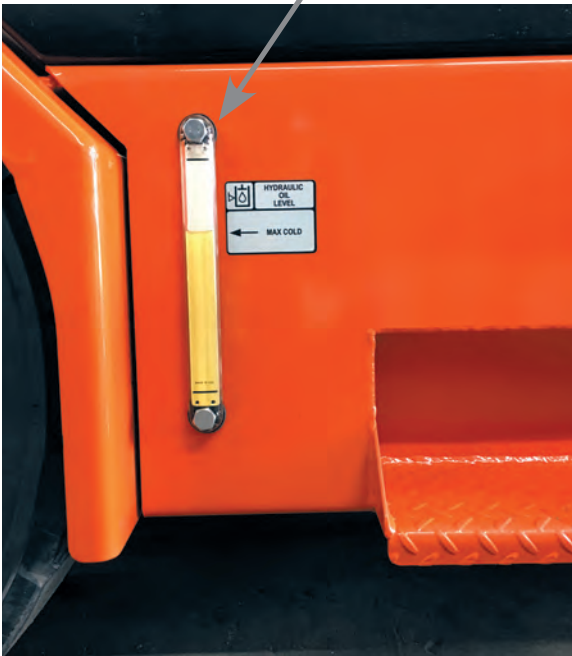
Hydraulic oil level
