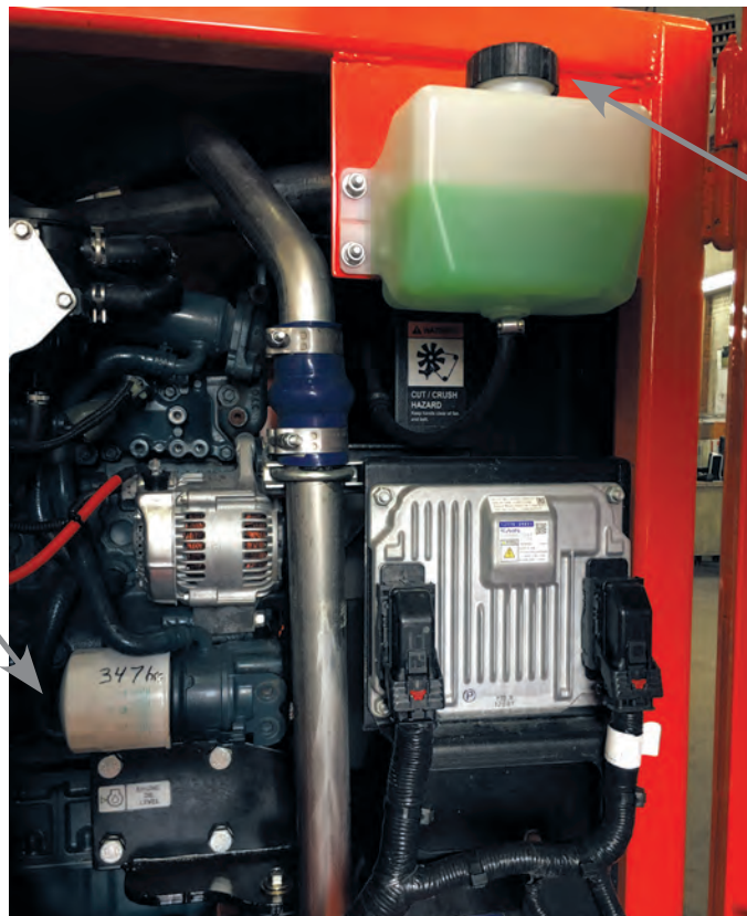
Check coolant level
