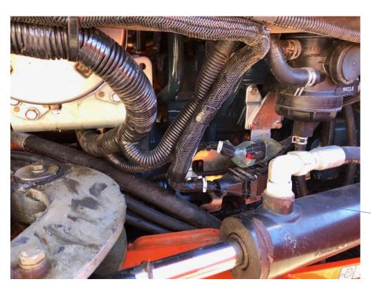
Inspect in this area on the back side of the harness
