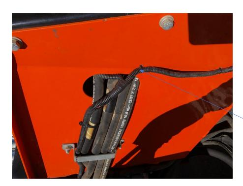
Cut into loom here to splice. This is the right side of the cab on the outside.
