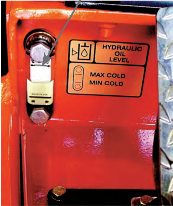
Hydraulic oil level
