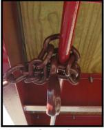
Picture shows chain loop being used to secure the binder to a tie bar beneath the trailer.
