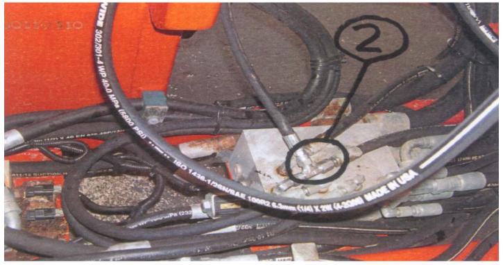
Step #4: Behind the hinge post for the fuel tank, you will find a plug on the side of the hydraulic pump. Attach the #4 hydraulic line from the 10,000 psi gauge to check the forward high pressure. Deadhead the machine against something solid and check with the rpms maxed out.
